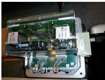
Figure II-8.2 A detailed view of the axle counter system with DIN plastic housing
