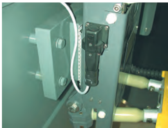
Figure II-12.4 Han® Q 5/0 in the Han® 3 A HPR housing
