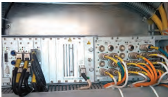
Figure II-7.2 Train control unit with Ethernet
