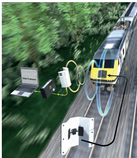
Figure IV-1 RFID System with reader, antenna and transponder from HARTING
