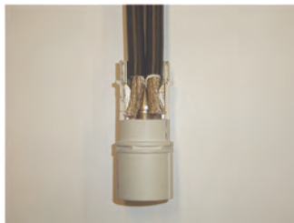
Figure VI-10.2 Doubled contacting on contact Han® HC Modular 350 of 2 cables each 25 mm 2 wire cross-section
