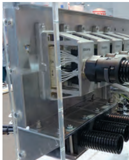
Figure II.-4.4 IP20 wagon coupling with modified housing
