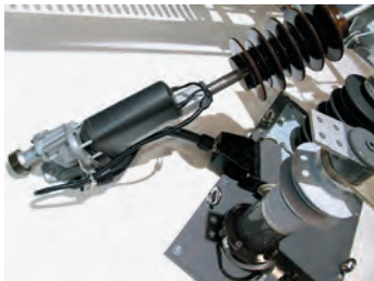
Figure II-12.2 Close-up shot connector Han® HPR on pantograph
