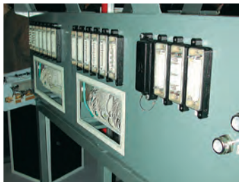
Figure II-10.4 Sub-floor container, back side with the HARTING Han® connectors
