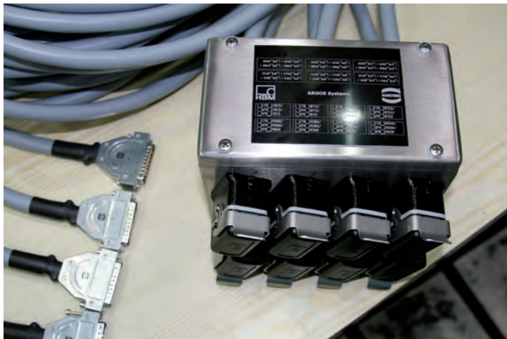
Figure VIII-5.1 Stainless-steel distributor box, Heavy Duty Connectors and pre-assembled D-Sub cables
