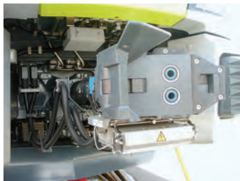
Figure II-13.1 Han® HPR interface between coupling unit and vehicle
