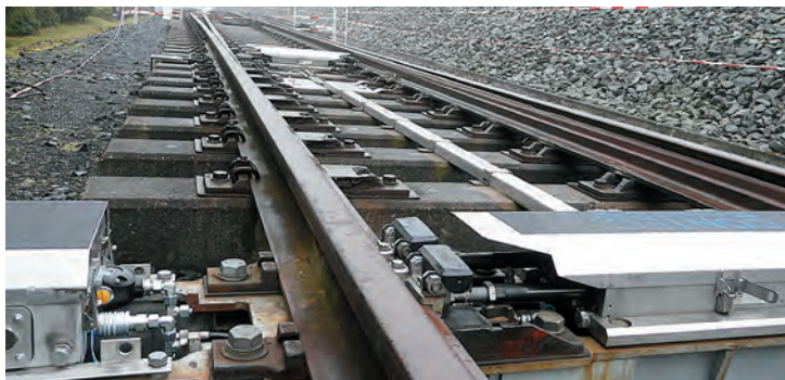
Figure II-8.3 Han-Yellock® on the CONTEC point drive
